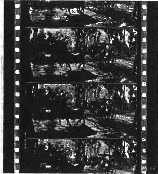
Fig. 2. Strip of 70 mm film. It has six magnetic sound-tracks, three on either side of the film. The wide black bands on the outside of the perforations carry two sound-tracks each; the narrower bands inside the perforations carry only one each. The height of the frame is equal to 5 perforations.
